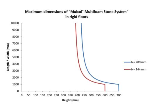
The maximum length (width) of the seal in rigid floors has to be calculated as follows:
