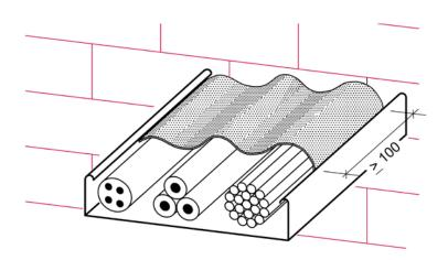
Step 2: Wrap the cables/ cable bundles and cable trays with "Mulcol ® Multifoam Wrap"
