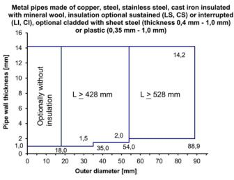
L measured from the surface of the penetration seal see ANNEX B-1 to C-3 of the ETA.
